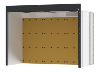
For the best aerodynamic stability, the front plates are rounded at the cabinet's open end. This design ensures uniform induction in the spray booth's opening, while preventing recycled paint vapors from escaping out of the premises and keeping the booth's sides cleaner.
